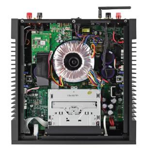
Inside is a linear power supply based around a large toroidal transformer, plus Class A/B power amps at left and right, attached to their heatsinks. At bottom (in the pic) is the auto-load (no tray) CD drive.
